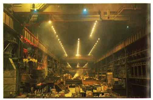
The British Steel Corporation at Ravenscraig has changed its lighting to 600W Solarcolour lamps from 1kW mercury, increasing the illumination by 20% and decreasing the lighting load by 40%.
