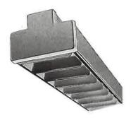
This low brightness louvre attachment is designed for use in areas where glare has to be reduced to a minimum. Due to its 'batwing' distribution the luminaires can be spaced further apart reducing installation cost.
